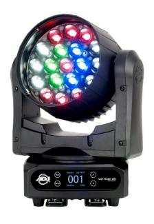
The Vizi Wash Z19 is a 380W professional moving head wash fixture with variable motorized zoom (10 ~ 60-degrees) and nineteen 20W Quad (RGBW / 4-IN-1) LEDs.
